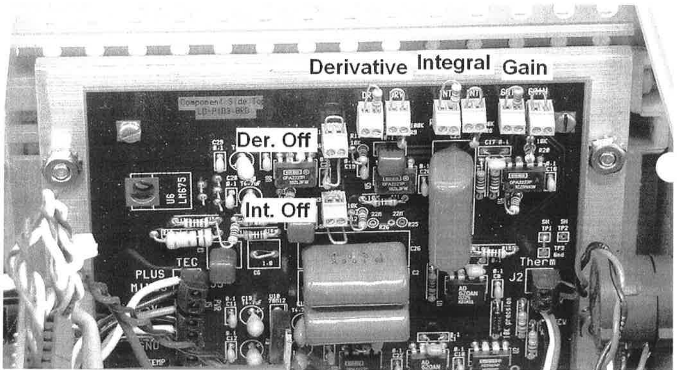
Figure 4: Picture of temperature control board showing terminal blocks
