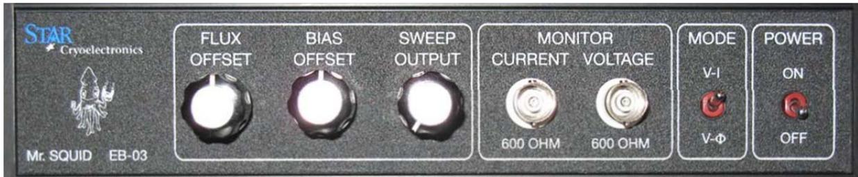
Figure 7: Front panel of the Mr. SQUID<sup>®</sup> electronic control box.
