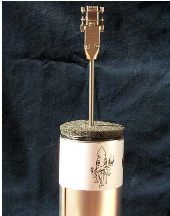
Figure 8 Mr. SQUID<sup>®</sup> probe inserted into the liquid nitrogen dewar.
